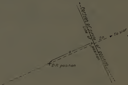
FIGURE 84.—Line of position.
